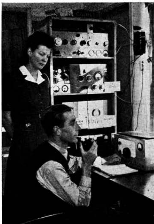
Eileen and Denis Heightman, G6DH, partners at one of the most outstanding amateur stations in the world with the gear that gave them their first 50 Mc/s. contacts with the U.S.A. and Egypt. The top shelf contains a 150 watt 7, 14 and 28 Mc/s. V.F.O. transmitter. Below is the transmitter used for 50 Mc/s. The modulator with two 809's in zero bias Class B is on the third shelf and beneath that is a 25 watt 3.5 Mc/s. transmitter. Power and grid bias supplies are also on the two bottom shelves with an automatic sender. A converted, 1154 relay used to change over aerial feeders, etc., is on the wall. The receiver is on the table.
